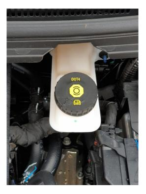
b. "The level must be between the minimum and maximum marks"
