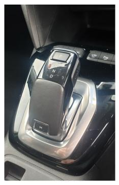
It has three buttons embedded in the gear stick. The "Park" button on the top, an Unlock on the upper right side, and the manual on the bottom.
