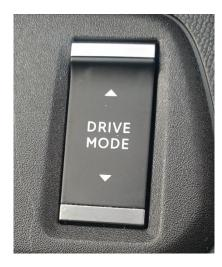
The car 3 modes: Sport / Normal / Eco. These different modes change the way the car applies power and times the gear changes.
